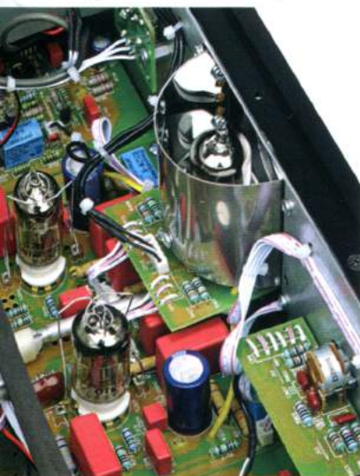
Behind the front panel window is an alloy reflector surrounding the 12AX7 input valve – seen at right.
