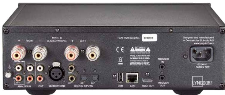
The limited space on the back of the 1120 has been used well; it can, however, quickly become quite crowded when using particularly thick cables.
