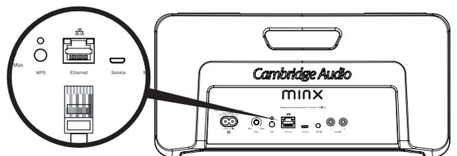
**Note:** Only connect the LAN port of the player to an Ethernet port that supports 10BASE-T or 100BASE-TX. Connecting to any other ports or jacks, such as a phone jack, can damage the unit. Now turn on your Minx Air.
