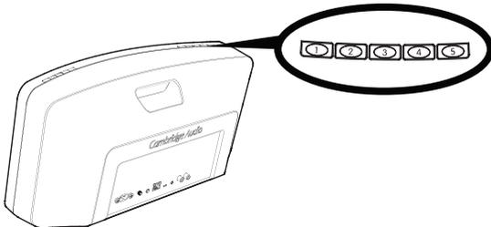
When a station is recalled in this way the
