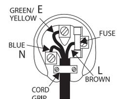
If a standard 13-amp (BS 1363) plug is used, a 3-amp fuse must be fitted or, if any other type of plug is used, a 3-amp or 5-amp fuse must be fitted, either in the plug or adaptor, or on the distribution board.
