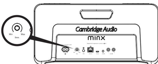
The Bass control can be found on the rear panel of the Cambridge Audio Air 100/200 Wireless Music System. Changing this setting allows the bass/low frequency response of the unit to be tailored to your taste and the acoustics of your room.
