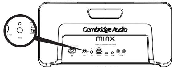
The WPS light on the rear of the Minx Air will flash orange > green > red for up to 2 minutes whilst the Minx Air looks for your router.
