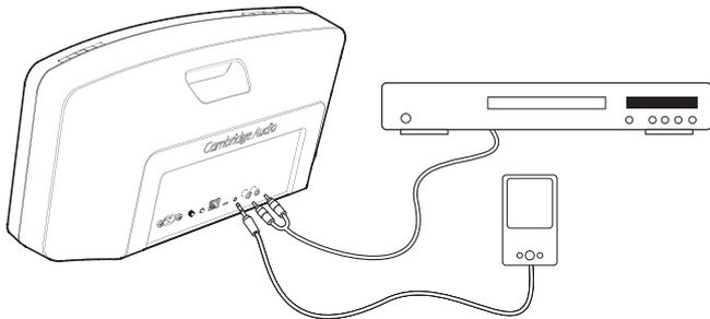
When the Minx Air is not streaming audio from Bluetooth, Airplay or Internet radio is automatically selects the analog audio inputs for playback.
